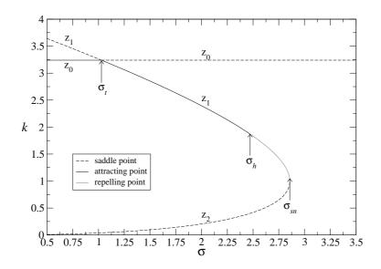
Figure 1: Local bifurcation diagram (stability of steady states).
